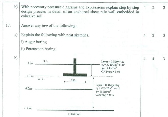
Consider shallow foundation in the figure failing under Local Shear Failure condition. Calculate net safe bearing capacity with a FOS 1.5 when Ground water level is at -1m elevation.
